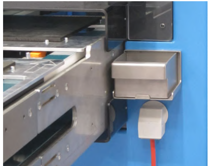
KVT 50-W90 - Page 46 Low profile 90 degree routing of a terminated cable from a control panel into the machine
