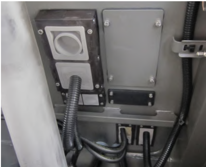
KEL-JUMBO 2 - Page 36 / KEL 24|x - Page 18 Routing of conduits and large cables between vehicle body and chassis
