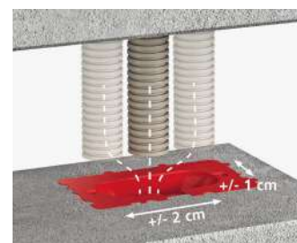
Good compensation of construction tolerances.
