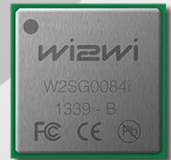
W2SG0084i - GPS Module based on SiRF Star IV™ with EEPROM
