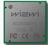
W2SG0021i - GNSS Module | GPS, GLONASS, QZSS, SBAS | based on SiRFstarV™
