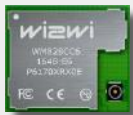
WM828CC6 - Dual Band Wi-Fi + Bluetooth 4.2 (Smart Ready / BLE) Combo Module with MHF4 IPEX connector
