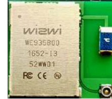
QFN-64 Footprint: 15 mm x 16.5 mm x 1.86 mm
