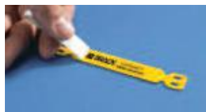
2. Place the label in the middle leaving space for sealing on all four sides of the label.
