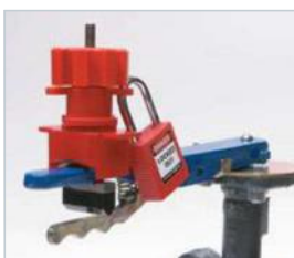
Clamp attaches to butterfly valve lever, preventing trigger handle from being squeezed. Valve cannot be repositioned
