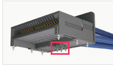
Localized press-fit control and power contacts eliminate the need for a secondary cable and connector
