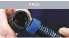
The FPAX fitting features a conduit seal to provide an IP rating up to IP69. This simply fits onto the end of the conduit before the fitting is connected to the conduit. To aid assembly moisten this seal. For a one piece fitting with an IP69 rating use Ultra™ (An FPA fitting cannot be uprated to IP69 with the addition of a seal). Pull back slightly to ensure the locking teeth mechanism has engaged with the corrugations.
