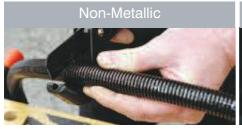
Non-metallic conduits to 34mm can be easily cut with Flexicon Conduit Cutters, part no. CC01. Use CC02 for sizes up to 67mm. Drop the blade into a corrugation and squeeze and twist until conduit is cut 50% through. Cut the remaining 50% without twisting to achieve a square cut.
