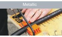
Metallic conduits should be cut with a fine tooth (32 TPI) hacksaw or bandsaw. Ensure you make a straight vertical cut. Our clamping vice, part no. BSB makes the use of a hacksaw much easier.
