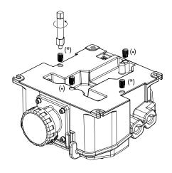
(\*): Inserts for horizontal fixing to bracket
