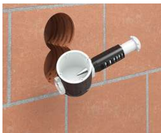
The flush-mounting fire-protection box provides 6 entry options for conduits up to M25 and cables up to \varnothing 11.5 mm.
