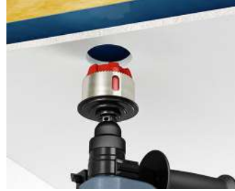
To expand existing installation openings from Ø 68 mm to Ø 74 mm using centering insert (Art. No. 1083-99).
