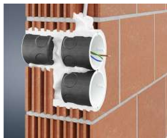
Fire protection is guaranteed with directly opposing installation and with less than the minimum remaining wall thickness.
