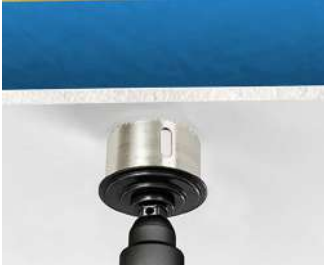
Make cut opening (e.g. with turbo cutter MULTI 4000 – Art. No. 1084-10).
