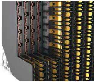
Staggered differential pair design with an embossed ground plane
