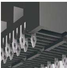
Staggered press-fit tails
