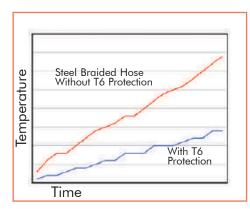
After long term exposure to extreme temp. (1,400°F) with the distance of 3/8" from the source of heat, T6 Thermashield remains flexible and resilient with no delaminating or breaking of the adhesive.
