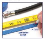
Measure the sleeving and mark the measurement with a pen or marker. Add an additional 38mm-51mm and cut the extended length of sleeving.
