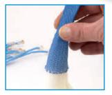
To install the sleeving over your application, just push the flared end over the ends of the wires and "walk" the sleeve down the length of the bundle from behind. Once the sleeving is in place, just run your hand over the applied sleeving to smooth it out.
