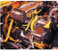
High thermal and chemical resistance and wide color/size selection make Flexo PET ideal for customizing and protecting the wires, hoses, and cables in custom and classic cars.
