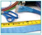
Measure the heatshrink tubing to length and cut with a scissor. The thickness of your bundle, as well as the desired final appearance, will determine the length of the tubing you cut. Generally, a piece 1 1/2" - 2" long will accommodate almost any need (such as this bundle of network cables). Single wires, or smaller bundles, require shorter pieces.
