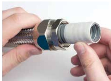
3. When using a conduit in a smooth coating - go to step 4. When using a conduit with vacuum coating apply the sealing couplings 66BTP on the head of the pipe to ensure the degree of protection IP. Note: Fold the coupling back on itself and make it fit on the conduit making sure that the inner spiral is inserted in the coils of the conduit. The ends of the conduit and the coupling must be aligned.
