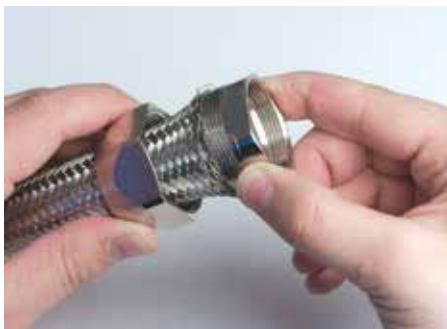
2. Install the intermediate body under the braid, after removing the tape. Firmly secure the nut and the intermediate body together, thus ensuring the locking of the braid.
