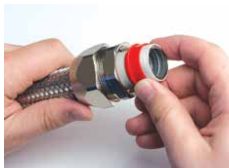
4. Insert the (nylon red) clamping sleeve with the truncated conical part facing towards intermediate body. Tighten the locking nut until it is fixed on the bushing.
