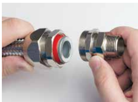
7. Insert all the elements in the body of the fitting and tighten the nut (with appropriate instruments) with torque suitable to maintain the IP degree of coupling. If necessary, insert the gasket (flat or O-ring) on the cylindrical male thread, until it stops.
